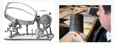
Figure: The phonautograph: a device that scratched sound waves onto a sheet of paper blackened by the smoke of an oil lamp.
