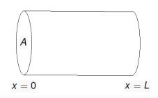
To understand the distribution of heat energy in the rod we consider the heat energy density e = e(x, t), i.e., the heat energy per unit length at position x and time t.
