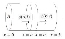
• Possible heat sources Q(x, t), i.e., the amount of heat energy per unit volume generated per unit time.
